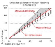
Surgic Pro calibration ensures outstanding safety because it minimizes deviations and ensures virtually no upward variations from pre-set values. As the graphs show, no calibration can be accurate without taking handpiece usage conditions into consideration.
